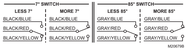
Fig. 6. Auxiliary switch wiring (S20 Series).
